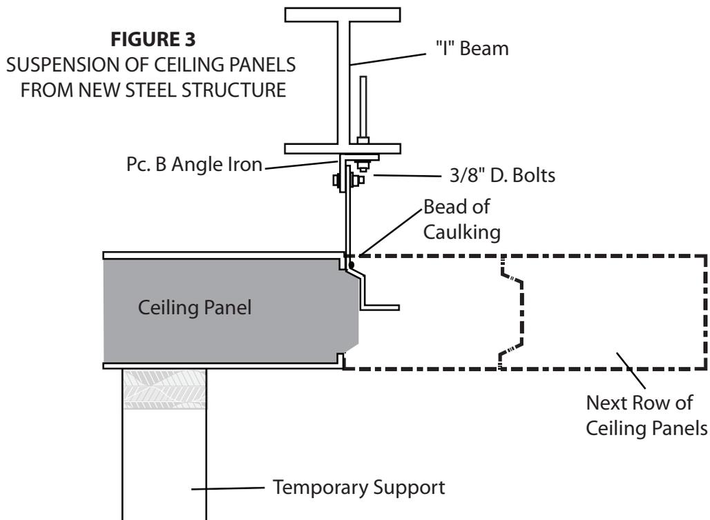
*Note: It is important NEVER to walk on top of a Bally ceiling that is not supported by interior steel or other temporary structural supports. Failure to support ceiling will cause joint failure and likely cause serious injury or death.*
